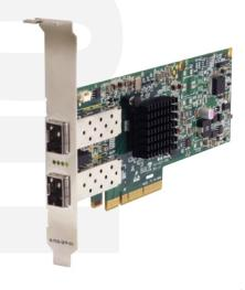
The N-TGE-SFP-01 is a PCle bus 2-port 10GBase-SR/LR SFP+fiber NIC that fully complies with IEEE 802.3ae standards. It provides up to 20 Gbps full duplex bandwidth capacity to support high-end servers. It is suitable for Data Center, SMB and Cloud computing applications. Two LED indicators (LINK and ACT) on the bracket will help to oversee the board link and activities status.
