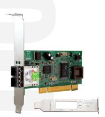
The Gigabit Ethernet NIC provides a 1000BASE-SX/LX fiber port, delivering fiber optic connectivity to the desktop for fiber rich LAN environments. With both standard and low profile form factors, driver support for most popular operating systems and PCI 2.2 plug-and-play capability, installation is a breeze in virtually any PC in your network.
