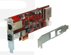
The N-GXE-POE-xx-01 Network Interface Card (NIC) provides connectivity to a secure fiber network while also delivering power to a PoE Powered Device (PD), such as a VoIP phone with a copper UTP interface. It fully complies with all IEEE 802.3z and 1000Base-X standards, providing up to 2000 Mbps full-duplex bandwidth capacity.
