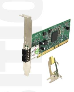
The Gigabit Ethernet NIC provides a 1000BASE-SX/LX fiber port, delivering fiber optic connectivity to the desktop for fiber rich LAN environments. With both standard and low profile form factors, driver support for most popular operating systems and PCI 2.2 plug-and-play capability, installation is a breeze in virtually any PC in your network.
